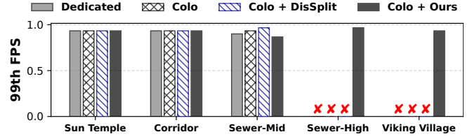
Figure 9: Normalized 99th FPS of different games with different deployment strategies. FPS values are averaged across multiple game sessions on the same hardware.
